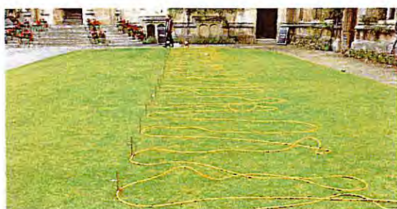
Illustration 4: An ERT probe array in use for a shallow stratigraphic study
