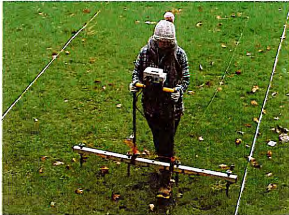
Illustration 2: Planar electrical resistance survey - typical configuration
